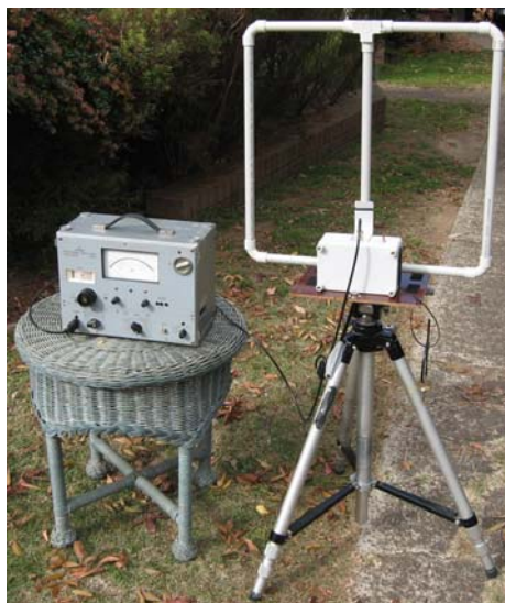
Figure 13: The field strength measurement system.
